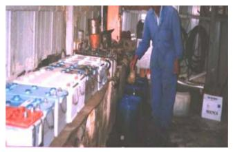
Figure 5 A partial view of storage battery repair unit in one of the enterprises. workers are engaged in routine activities without personal protective equipment, poor ventilation and full of dust.
